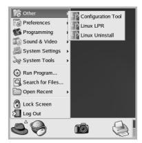
You can also access the Linux Printer Configuration window by typing "linux-config" in the Terminal screen.
